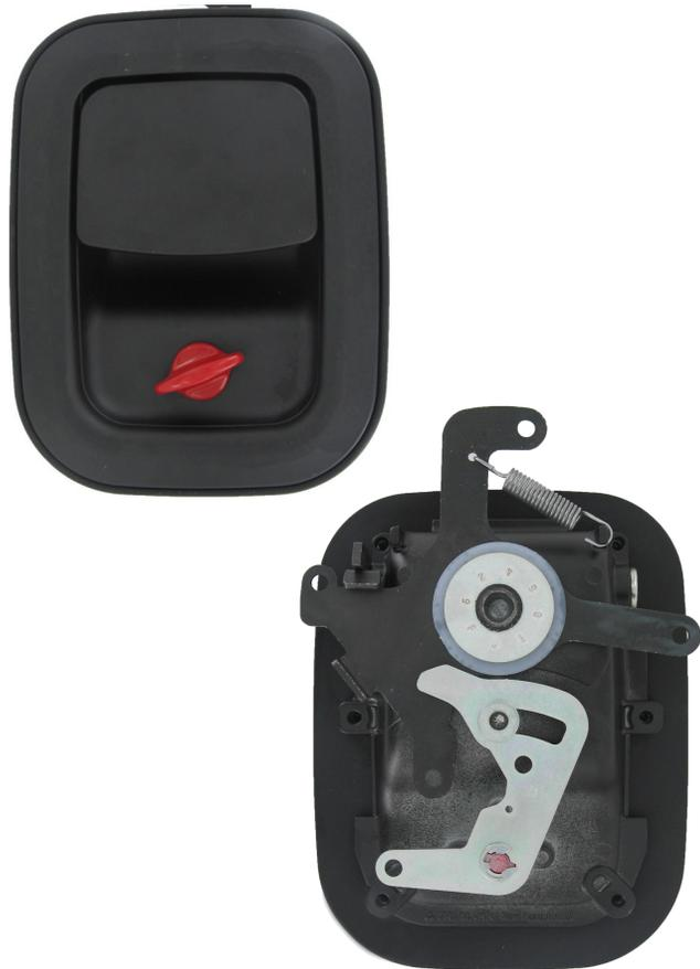
This flush mounted paddle handle with inside lock knob is a redesign of our popular 030-0860 Flush Mounted Paddle Handle. With a modernized look, it can be used in FMVSS 206 (ECE R11) applications, is power lockable and features a four point pivot plate and lock cam actuation.
